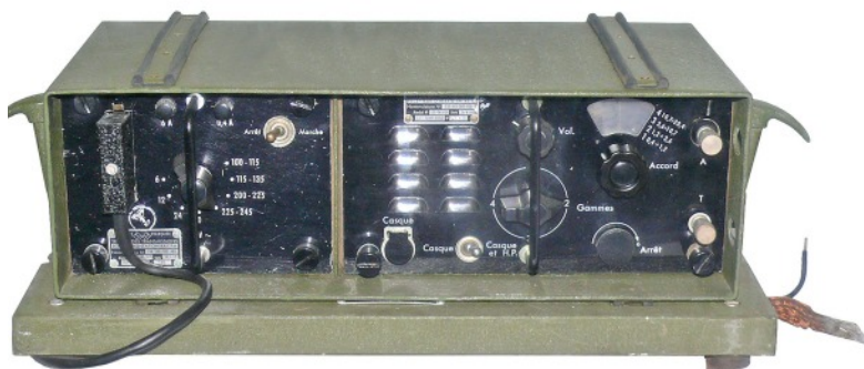
RR-49A receiver and associated BA-119 power supply unit in original metal enclosure (above and below).
