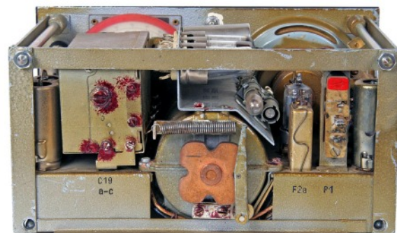
Rear view of RR-49A receiver showing the rotating turret coil unit in the centre.
